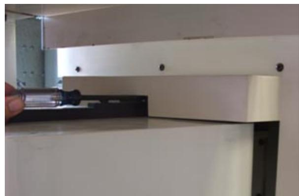
Figure 2: Using a long screw driver, manually bring the tool changer to the spindle by pushing the upper Geneva Arm
