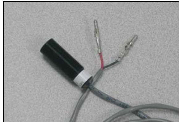
Figure 2: ELE-1202 Magnetic Reed switch
